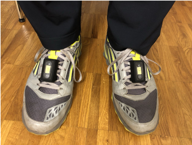
Figure 1: IMU sensors that are attached to the laces at the top of shoes to measure spatio-temporal gait parameters.
