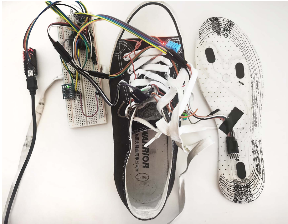
Fig. 2. The hardware prototype: a Converse-type shoe with low-level integration. We use breadboard prototyping with an Arduino Nano that streams the data via USB to a portable computer. Different to the previous version of ShoeTect [6], we waived on using the data gathered by the microphone and humidity sensor, although the sensors are still plugged. We believe the data not to be very meaningful for our activities.
