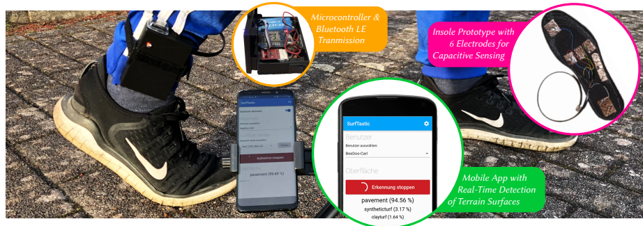
Fig. 1. Demonstrating SurfSole: The insole prototype, consisting of 6 copper electrodes, and a small box of electronics is worn on the right foot, while our mobile app "SurfTastic", running on an Android Smartphone detects the current terrain surface one is walking or running on.
