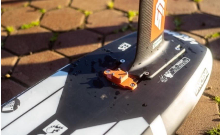
Fig. 3. Arduino Nicla Sense ME mounted to the bottom of the hydrofoil board.
