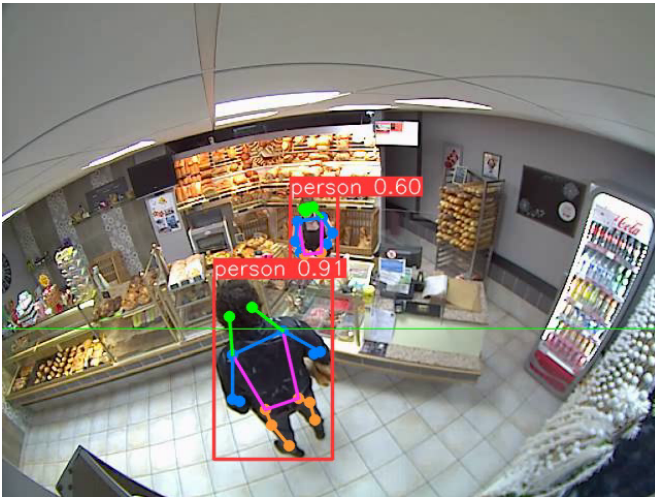
Figure 9: Example of pose estimation in the CCTV footage
