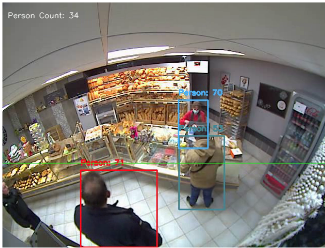
Figure 8: Example of object detection and tracking with bounding boxes in the CCTV footage
