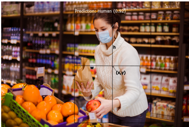
Figure 2: Bounding box example with predictions (x, y, w, h) and class label. Photo: Colourbox.com
