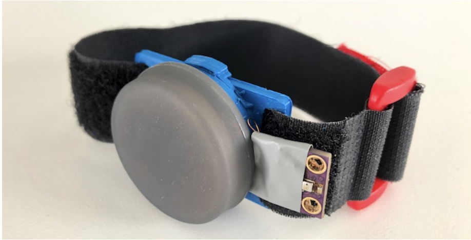
Fig. 2: Our prototype consists of a Puck.js with the attached BME280 sensor. A custom 3D-printed enclosure can be mounted on the wrist using the wristband.
