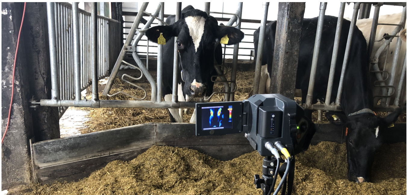
Figure 1. Contactless vital data assessment by thermal images.
