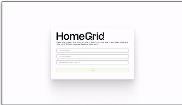
Figure 3: Access Point interface to setup the WiFi Credentials and device name.
